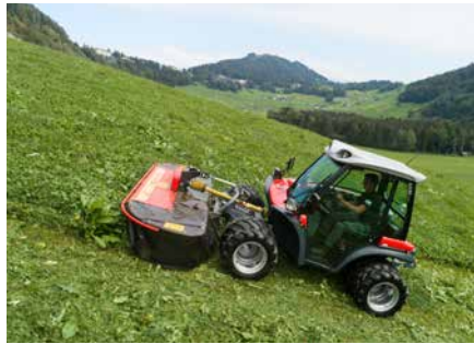
1. Gravity point is close to tractor for stable, safe operation on steep slopes.
