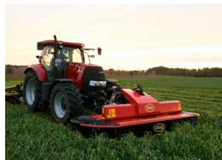
By switching driveline pulleys changing from standard PTO speed of 1000 rpm to 750 rpm is possible.
