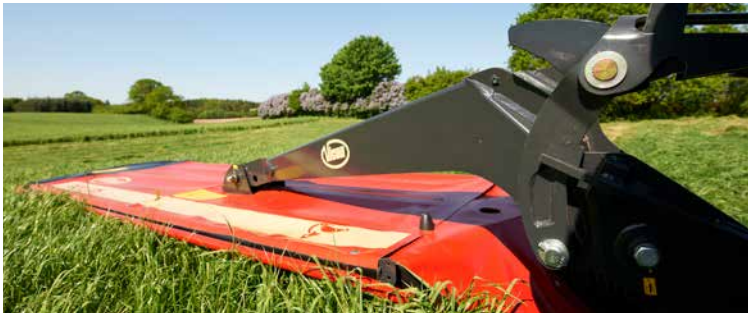
The centre suspended design enables fast and precise adaptation to ground contours.
