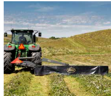
To avoid driving on mown crop, a swath forming kit is optionally available for EXTRA 436H and 440H.
