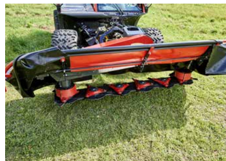
6. Six counter-rotating discs, each with 3 knives ensure excellent cutting performance.
