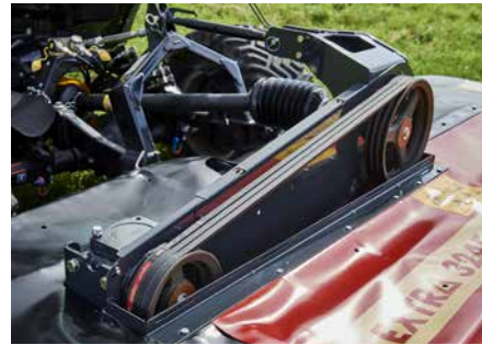
2. Switching between either 540 or 1000rpm is easy done by just swapping pulleys.
