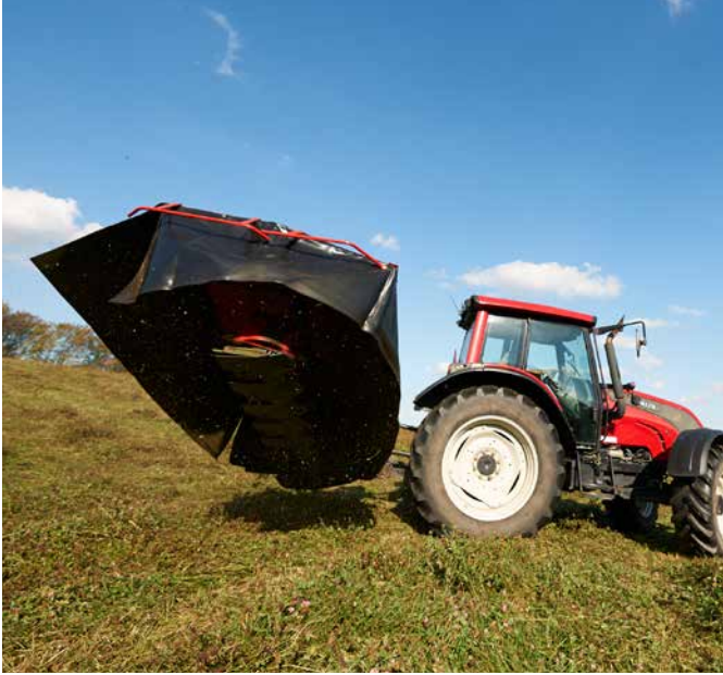
Lifting on headlands via a hydraulic cylinder.
