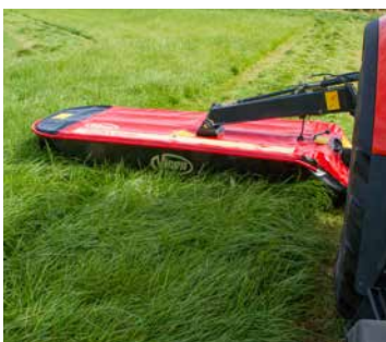
The machine can be operated at an upwards or downwards angle of 15°.
